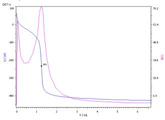
Fig. 1: Potentiometric determination of TAN (blue = titration curve, pink = ERC)
