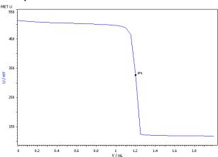
Fig. 2: Photometric determination of TAN
