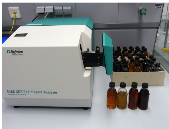
Figure 1. XDS RapidLiquid Analyzer and lubricant samples.
