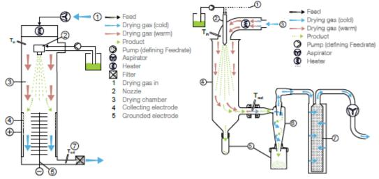
Figure 1 Functional principle of BUCHI Nano Spray Dryer (left) and conventional spray dryer - BUCHI Mini Spray Dryer B-290 (right).
