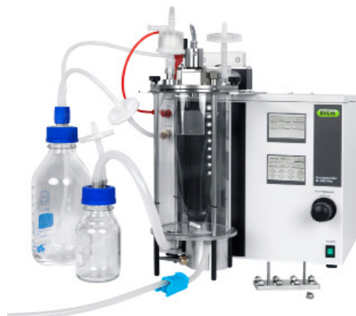
Figure 3: The standard set up of the BUCHI Encapsulator model B-395 Pro with sterile reaction vessel in place.
