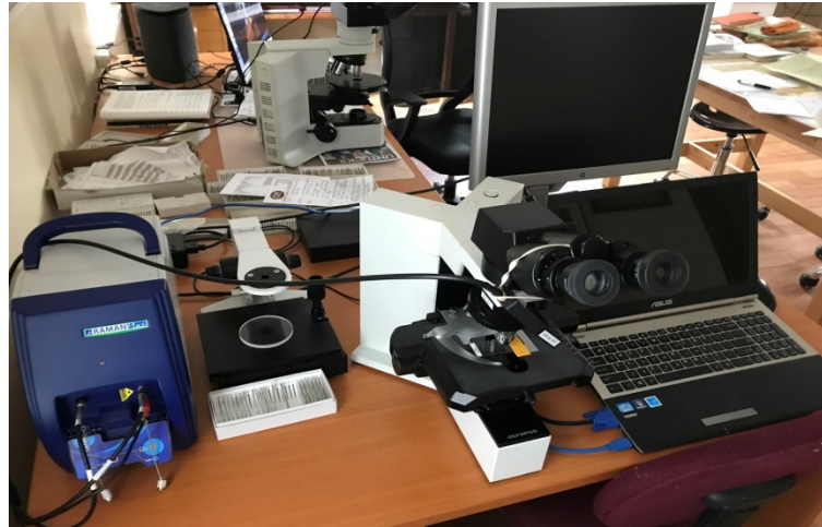
Figure 2. Photograph of the B&W Tek i-Raman Plus Raman system (left) interfaced with an Olympus polarizing microscope (center) as described in the text. Desk is 48 inches wide.
